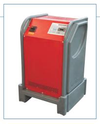
The 3750 Pulpress Series of microprocessor controlled pressurisation units are designed to make up any losses due to system leakage and to maintain the initial system design fill-pressure in sealed LTHW, MTHW or Chilled Water systems, and all types of systems as set out in BS7074 Parts 1, 2, and 3. They are ideal for domestic or industrial premises. 3750 Pulpress units are designed for applications where there is a need to pressurise and provide make-up for sealed systems within a building.
